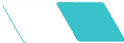
Figure 1 LIQOSEAL® with an adhesive white foam layer and blue sealing layer - schematic drawing
